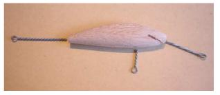
Next, **glue in the bib**. Use a piece of wire to coat the inside of the bib slot with glue. Cover the lower section of the bib (both sides) with glue. Align the centre line of the bib with the centre line cut on the lure. Push the bib into the slot and sight along the lure to make sure the bib is sitting straight. Clean off excess glue and fill the edges of the bib slot, if necessary.
